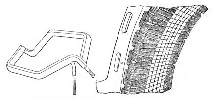
FIG. 61. Machine-formed coil for alternator armature, bent to permit overlapping.
